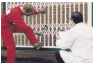
SecuroGuard 1001 undergoing a simulated attack test
