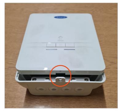
Remove Genesis control panel cover by pushing the cover up.
