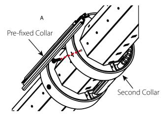
**IMPORTANT:** When attaching the collars, make sure that the fixing has <u>fully engaged</u> with the pre-punched hole on the axle (see **Drawing B**).
